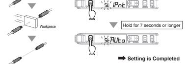
Incident light level setting: Adjust the max. incident light level on Step 1 as the power tuning level. Threshold setting: Set to the middle between max. and min. incident light levels on Step 1.
